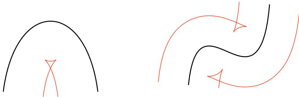
(a) Offsets of a convex curve.
